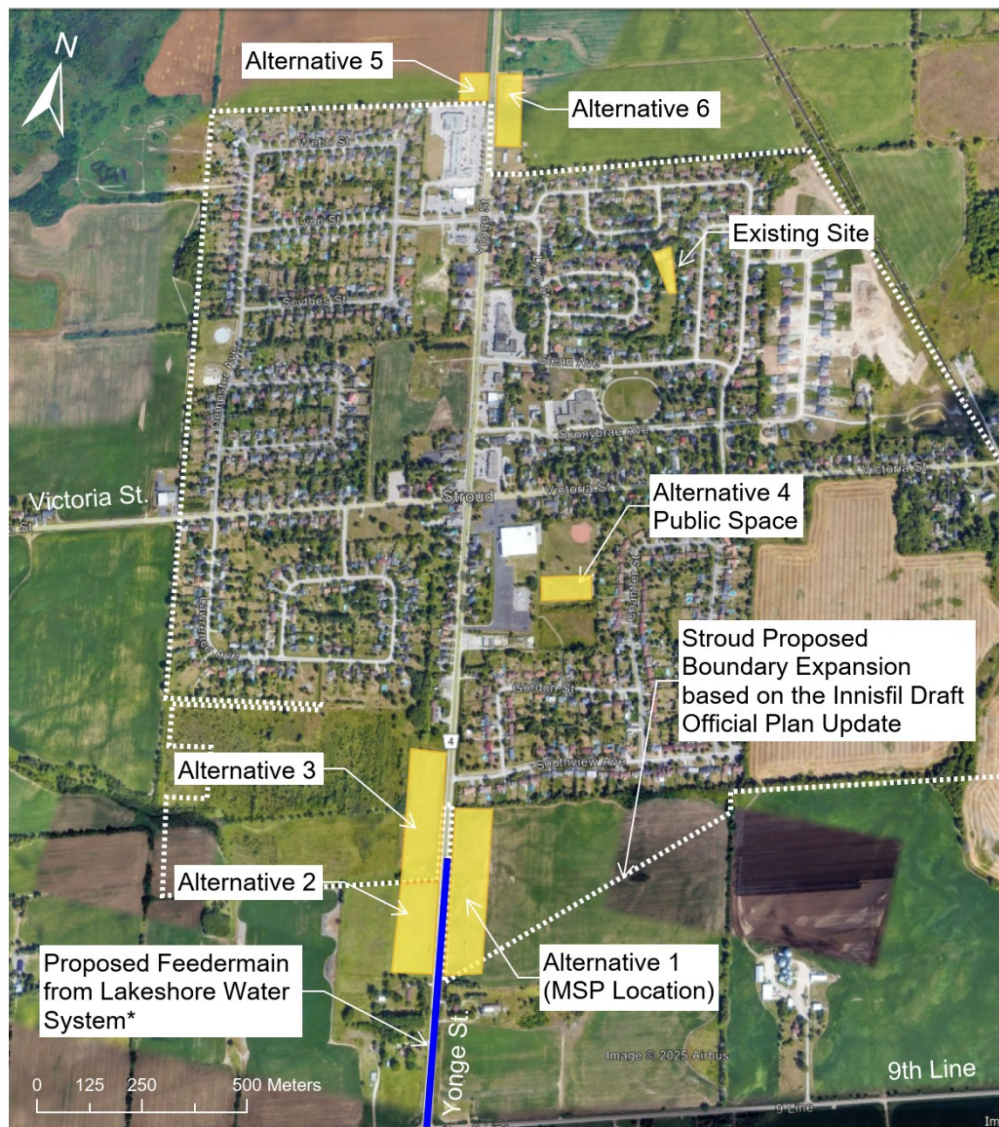
Figure 4.1 – Alternative Sites for the Water Storage Facility and Booster Pumping Station (if required)
